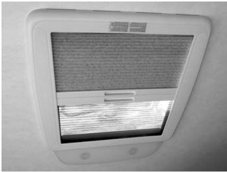
Fig. 116: Example of a skylight combination blind
