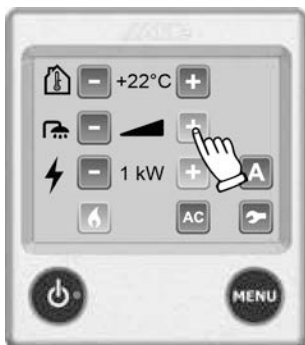
Fig. 150: More hot water
