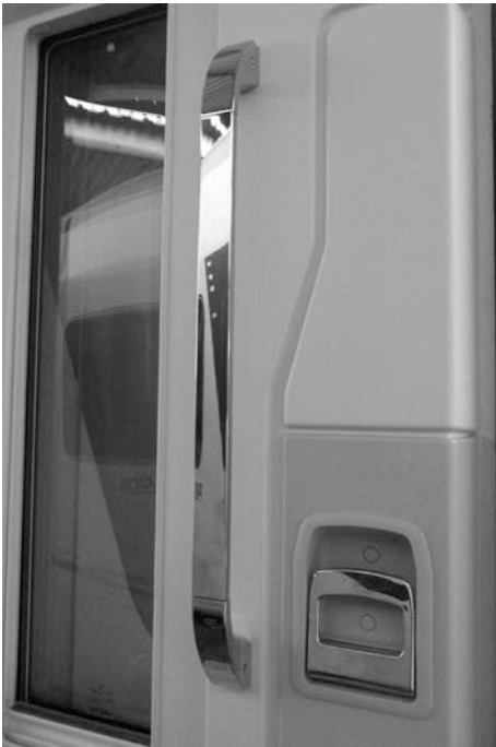
Fig. 18: Interior door with grab bar and handle
