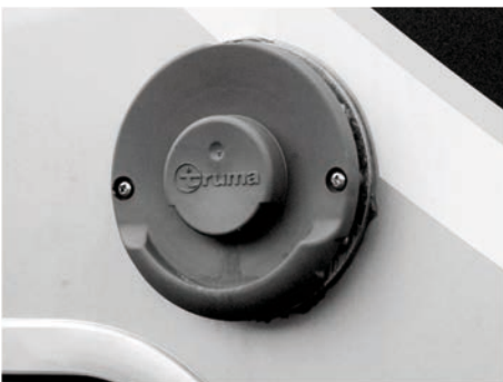
Fig. 80: Wall exhaust stack
