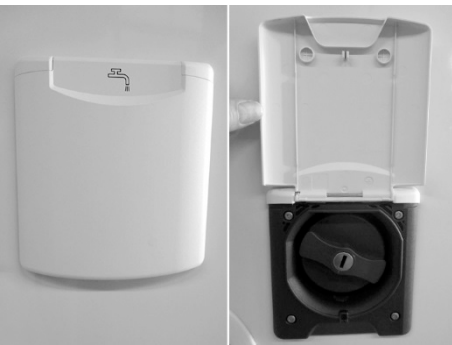
Fig. 21: Fresh water intake port
