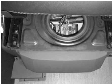
Fig. 7: Interface module under the driver's seat
