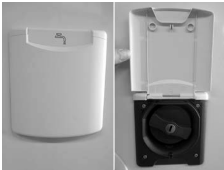
Fig. 97: Fresh water intake port
